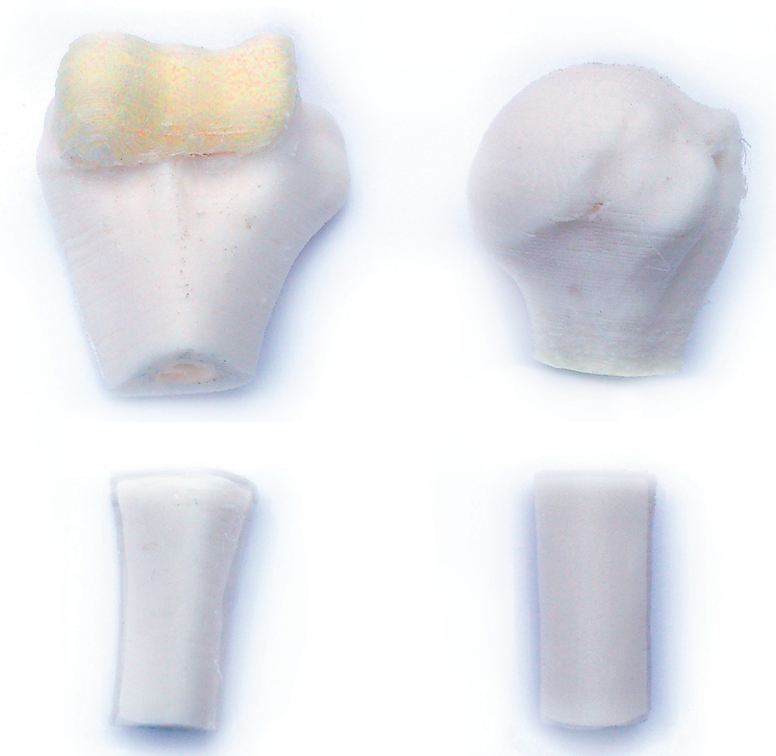
Figure 5. 3D printed prototype phantoms. Top row: Distal (left) and proximal epiphysis with bone, cartilage, and marrow analogues. Bottom row: Corresponding sections of diaphysis.
